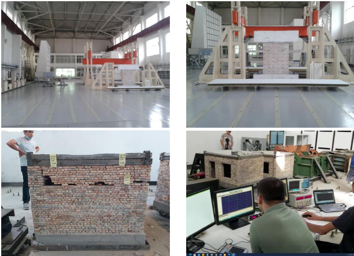
Figure 1. Preparation and shake table testing of unreinforced masonry assemblages at TTPU
