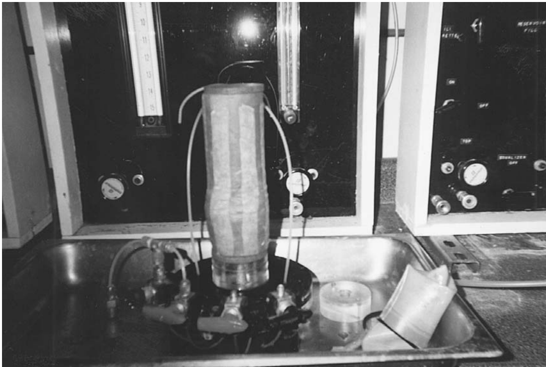
FIGURE 3.26 Bulge-type failure condition of the soil specimen.
