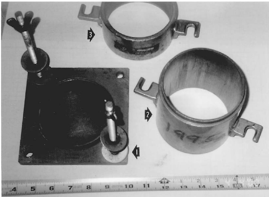
FIGURE 3.45 The compaction apparatus consisting of three parts: (1) base plate, (2) compaction mold, and (3) the top collar.
