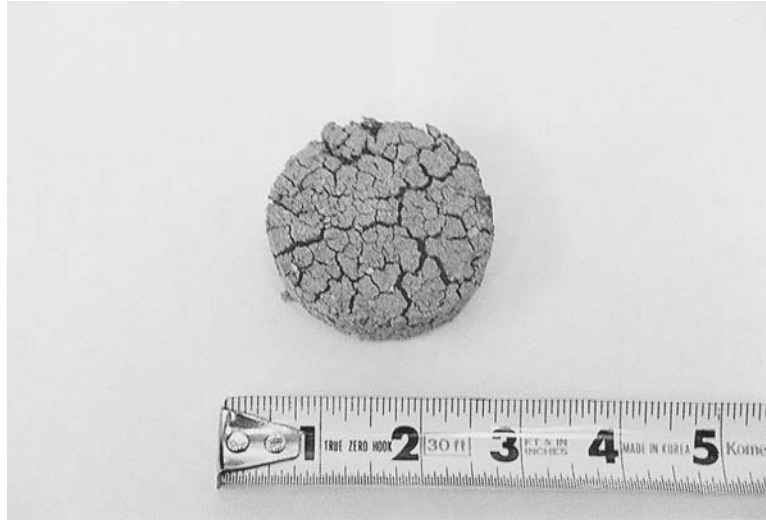
FIGURE 9.18 Specimen of desiccated Otay Mesa clay.
