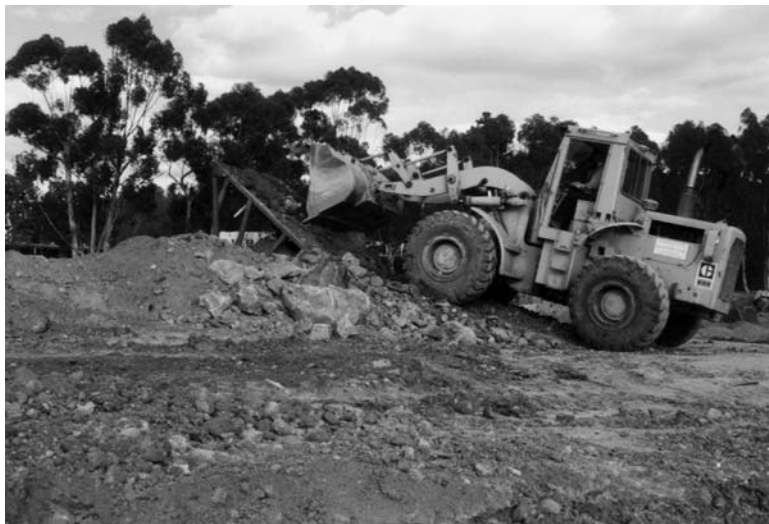
FIGURE 15.6 A loader is in the process of depositing material on top of the screen in order to separate the large size rock fragments.
