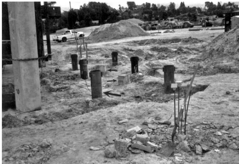
FIGURE 16.32 Pile load test. The small arrows point to the prestressed concrete piles that will be subjected to a load test. The large arrow points to one of the six anchor piles.
