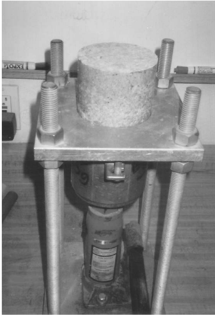
FIGURE 3.51 The compacted soil is in the process of being extruded from the compaction mold.
