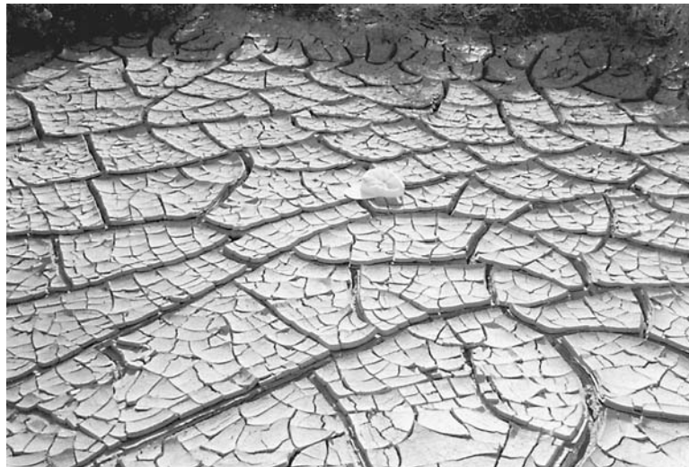
FIGURE 9.17 View of a deposit of desiccated clay located in Death Valley, California. Note that the hat in the center of the photograph provides a scale for the size of the desiccation cracks.
