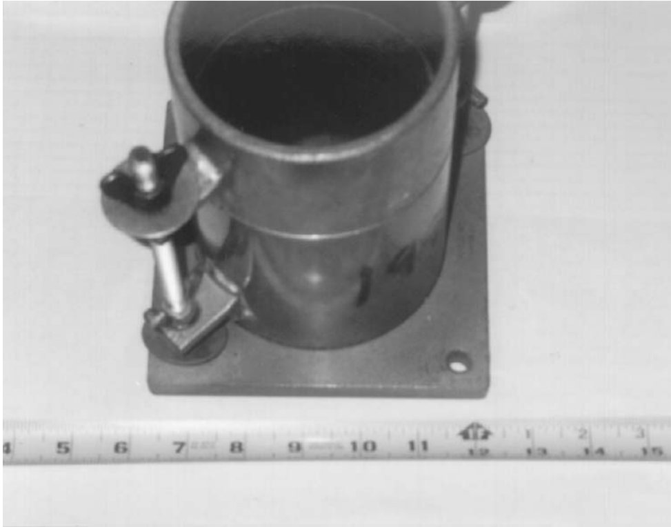
FIGURE 3.46 The compaction apparatus in an assembled condition.
