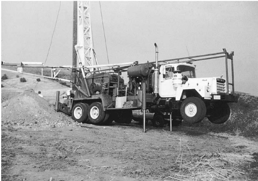
FIGURE 2.4 A flight auger drill rig (top) and a bucket auger drill rig (bottom).
