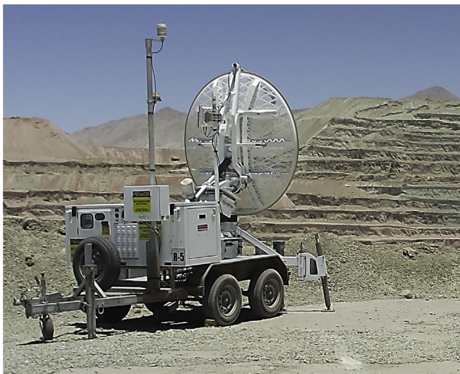
Fig. 27. Radar equipment for monitoring slope displacements.
