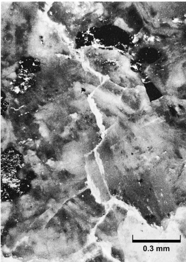
Fig. 6. Crack path in a specimen of Witwatersrand Quartzite from a deep gold mine in South Africa, sectioned after uniaxial compressive loading to about 75% of the uniaxial compressive strength.
