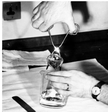
(e) Rubber components mixed. Pot life 5 min.
