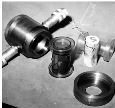
(h) Severely deformed specimens may require dismantling of cell.
