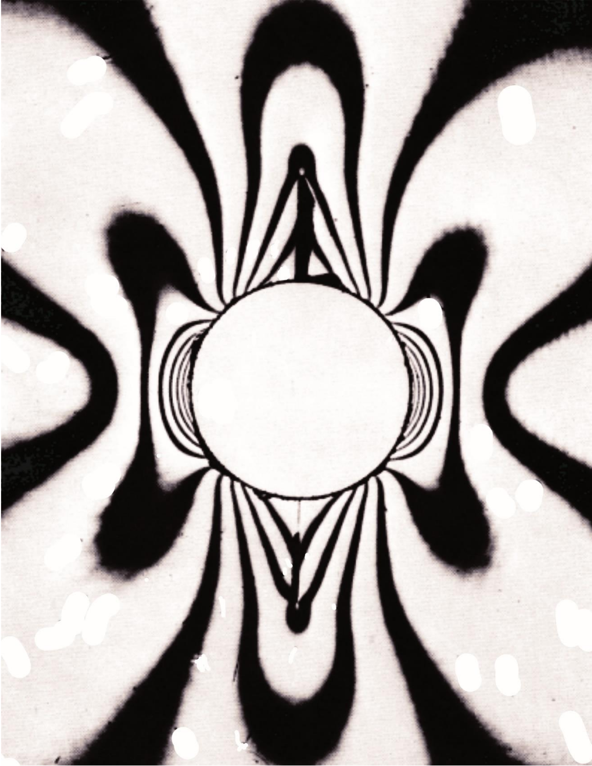
Figure 4. Photoelastic pattern in a glass plate model containing a central circular hole from which vertical tensile cracks have propagated.
