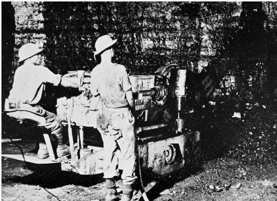
Figure 8. A universal coal cutter being used to prepare large scale coal specimens.
