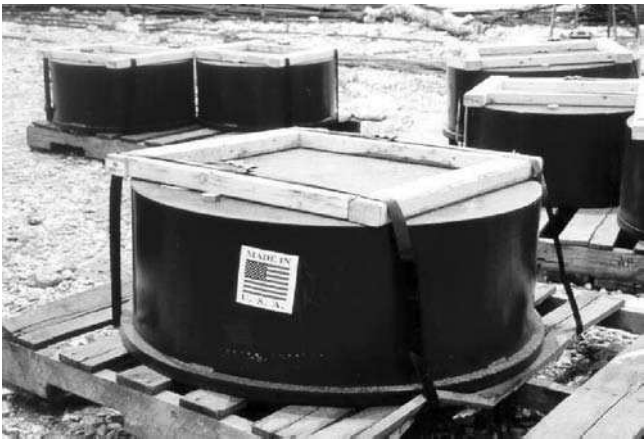
FIGURE 9.31 Osterberg O-cell. (Courtesy of Load Test, Inc.)
