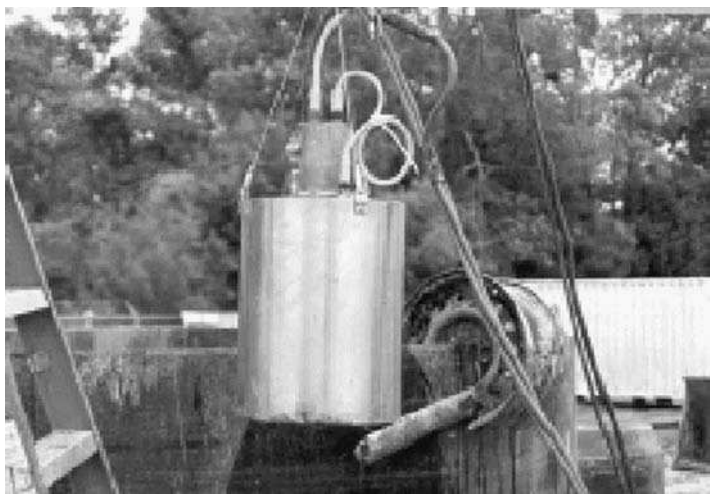
FIGURE 9.50 Equipment used for sonic echo test (left), impact hammer struck on shaft head (right). (Courtesy of Applied Foundation Testing, Inc.)
