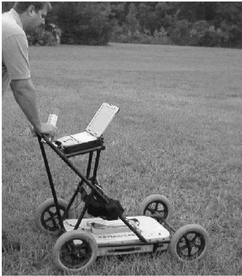
FIGURE 2.4 GPR field device. (Courtesy of Universal Engineering, Inc.)
