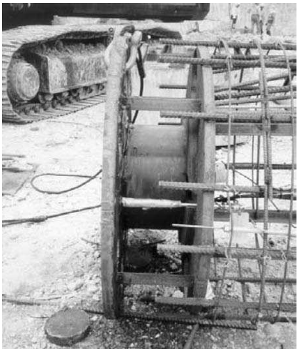
FIGURE 9.32 Osterberg cell being set up for load testing. (Courtesy of LoadTest, Inc. www.loadtest.com .)
