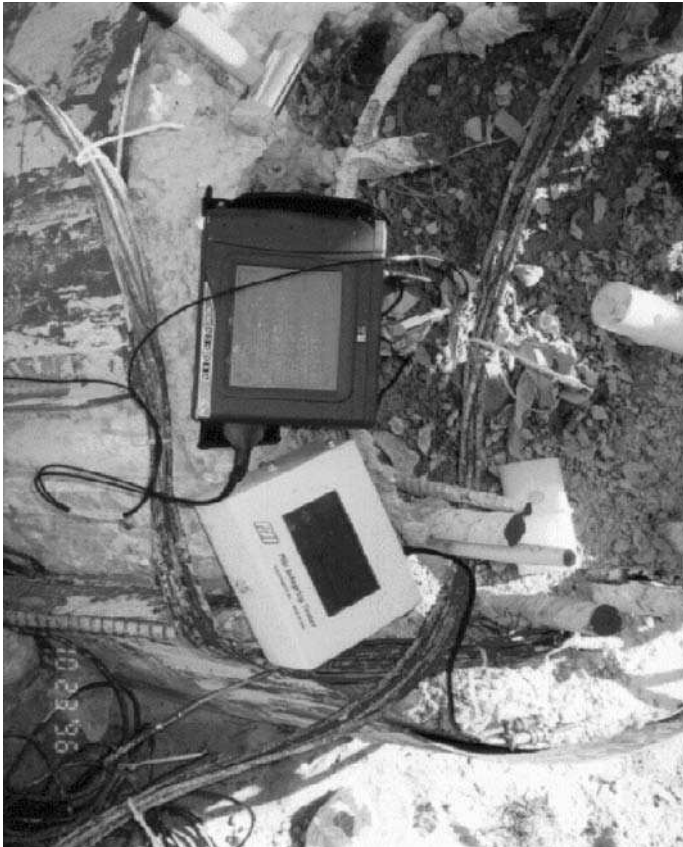
FIGURE 9.52 Miniature shaft inspection device. (Courtesy of Applied Foundation Testing, Inc.)
