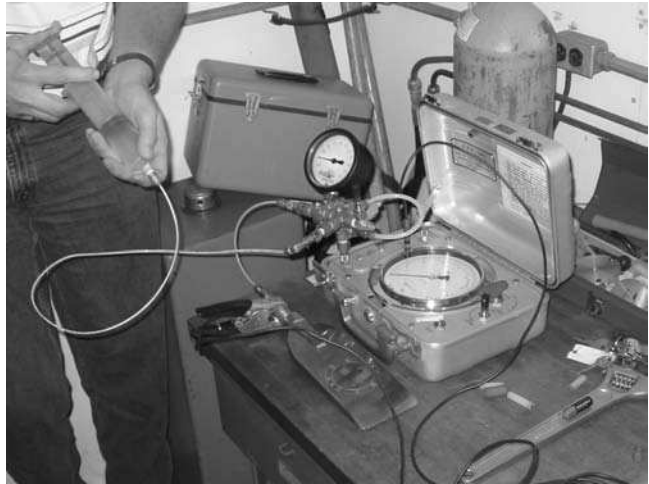
FIGURE 2.25 Calibration of the flat plate dilatometer. (Courtesy of the University of South Florida.)
