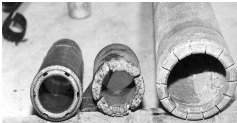
FIGURE 2.14 Cutting bits used by Florida Department of Transportation District I.
