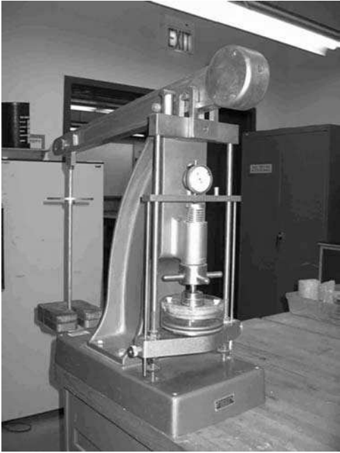
FIGURE 1.17 Laboratory consolidometer apparatus. (Courtesy of the University of South Florida.)
