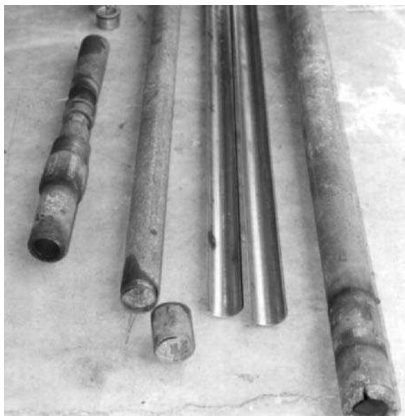
FIGURE 2.12 Triple-tube core barrel components.
