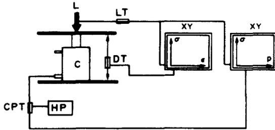
Fig. 2. A schematic diagram of the test equipment.
