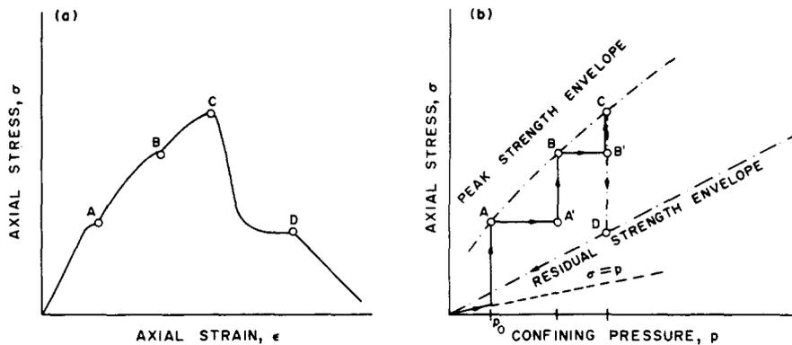
Fig. 4. Multiple failure state triaxial test: (a) The axial stress–axial strain curve; (b) the axial stress–confining pressure curve.
