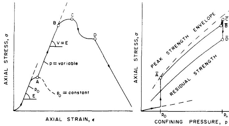
Fig. 5. Continuous failure state triaxial test.
