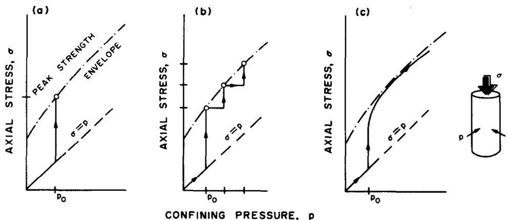
Fig. 1. Different triaxial test types: (a) Type I—individual test; (b) Type II—multiple failure state test; (c) Type III—continuous failure state test.
