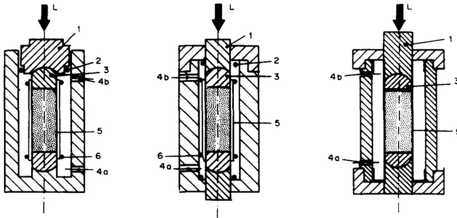
Fig. 3. Three possible designs for triaxial chamber.
