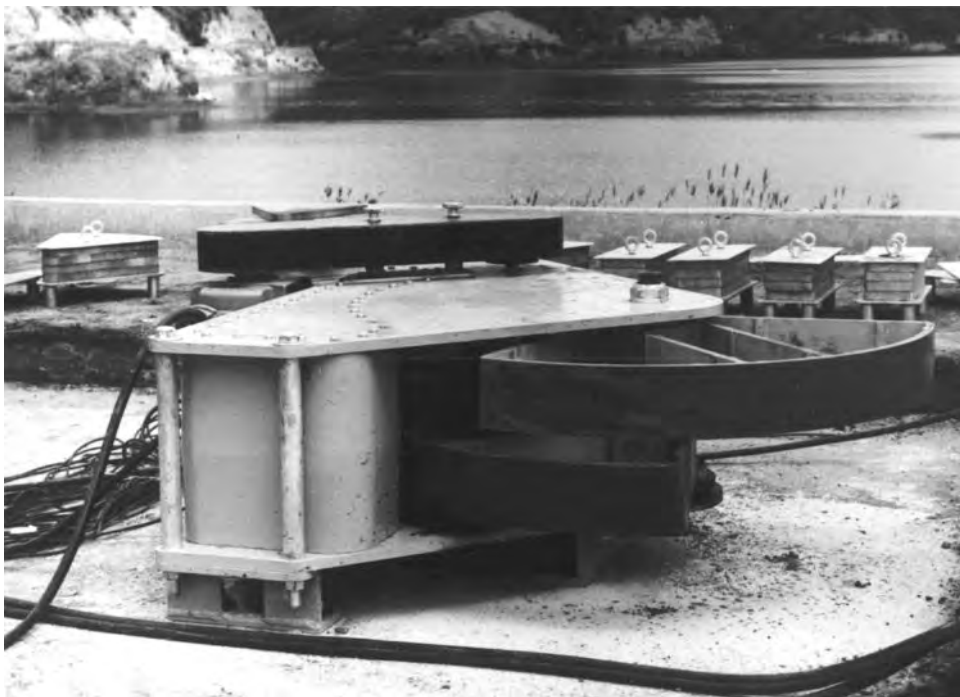
Figure 3.3.1 Counterrotating eccentric weight vibration generator.
