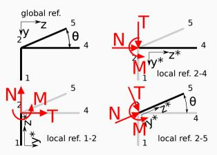
The components of resultant  $R_j$  are  $T_j$ ,  $N_j$  (local reference) and  $V_j$ ,  $H_j$  (global reference). Moment  $M_j$  is the same in both systems. Similar transformation for  $v_j$  and  $w_j$  (rotations do not change)
