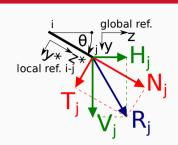
To move from local to global reference frame, the rotation matrix  $N_e$  is introduced:
