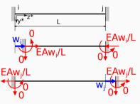
The displacement w of one end is applied and the corresponding reactions are calculated (local frame):
