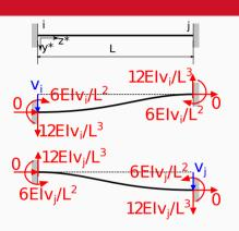
The displacement *v* of one end is applied and the corresponding reactions are calculated (local frame):
