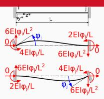
The rotation of  $\varphi$  of one end is applied and the corresponding reactions are calculated (local frame):
