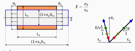
• Poisson's ratio  $\nu$ : ratio between transversal and longitudinal strains:
