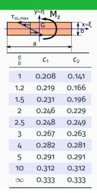
For cross section composed by N rectangles with sides equal to  $a_i$  and  $b_i$  with  $\frac{a_i}{b_i} \to \infty$  (i.e.,  $c_1 = c_2 = \frac{1}{3}$ ) it is:  $\tau_{zs,max}^i = \frac{M_z}{l_t} b_i$
