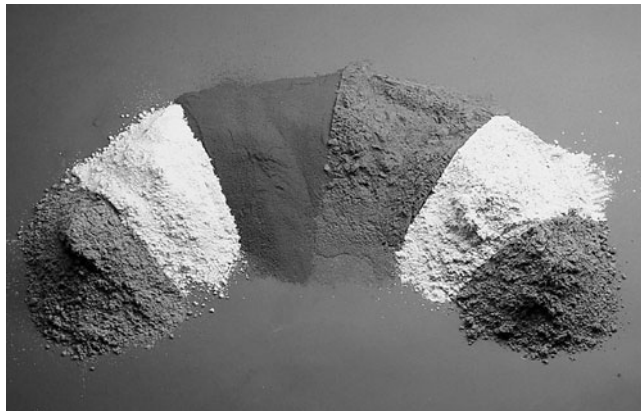
FIGURE 2.2 Supplementary cementitious materials. From left to right: fly ash (Class C), metakaolin, silica fume, fly ash (Class F), slag, and calcinated shale. (Courtesy of the Portland Cement Association.)
