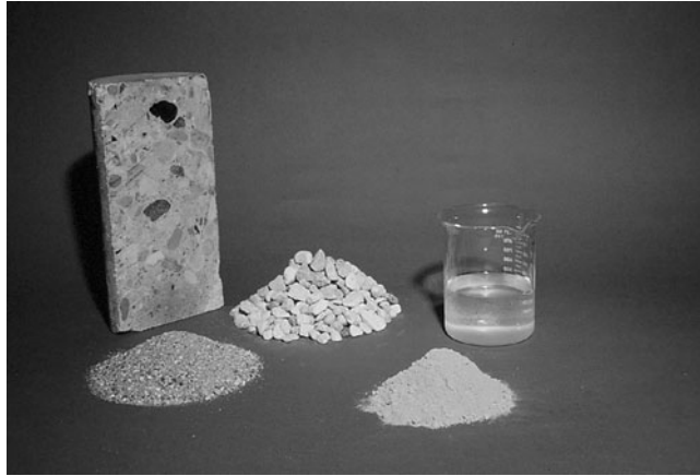
FIGURE 2.1 Concrete components: cement, water, fine aggregate, and coarse aggregate. (Courtesy of the Portland Cement Association.)
