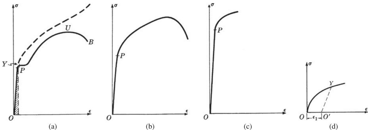
Fig. 1-3 Stress-strain diagrams.
