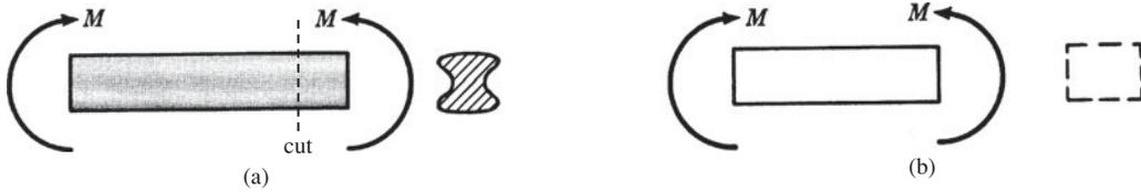
Fig. 7-2 A beam in pure bending.
