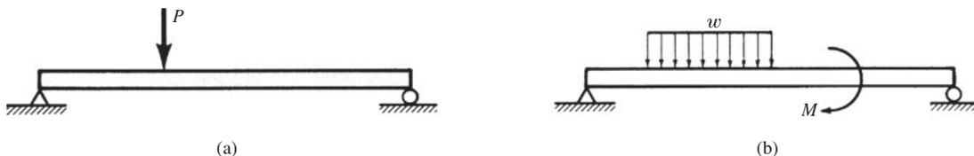
Fig. 6-2 Simple beams.
