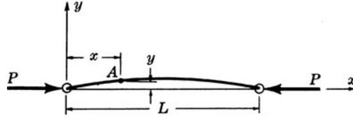
Fig. 10-2 The nomenclature used to derive  $P_{cr}$
