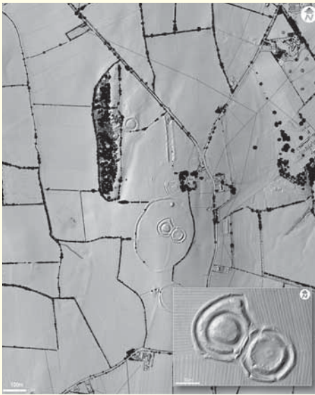
Fig CS11.1 Plan view of the DSM generated for the Hill of Tara from FLI-MAP data at approx. 60pts/m 2 (©The Discovery Programme).
