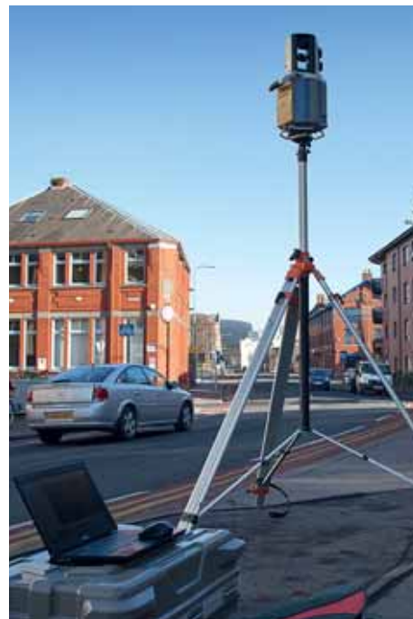
Fig 34 Laser scanning from an extra tall tripod (courtesy of Nick Russill, TerraDat).
