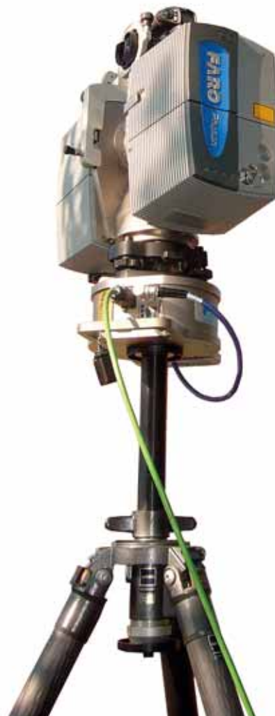
Fig 17 (below) A phase-comparison scanner (courtesy of Russel Geomatics).
