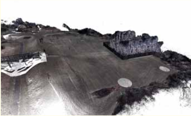
Fig CS8.2 Registered scan data showing the castle and surrounding earthworks, now a public park.
