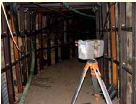
Fig CSI.1 (above) Faro LS880 protected for scanning.
