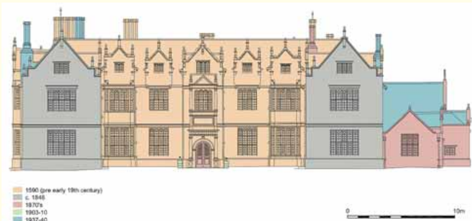
Fig CS7.2 (above) CAD drawing of the north elevation. Fig CS7.3 (below) Phased CAD drawing of the south elevation.
