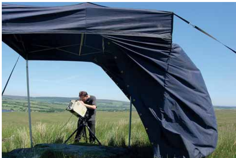
Fig 13 Triangulation laser scanning of rock art, on site with a canopy to reduce the influence of bright sunlight (courtesy of Tertia Barnet)
