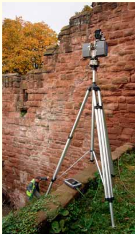
Fig CS12.1 FARO Photon scanner on tall tripod and the Chester city walls.
