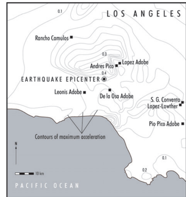
Map of Los Angeles, showing locations of historic adobe structures, the quake's epicenter, and contours of maximum acceleration. A map like this was used in planning site visits to the affected area. Drawing: Steven Rampton.
