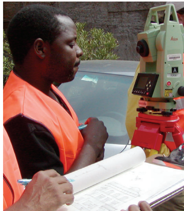
The author using a total station theodolite. The total station and its onboard computer calculate the position of a point through trigonometry by recording the horizontal and vertical angles and distance. Photo: Rand Eppich.
