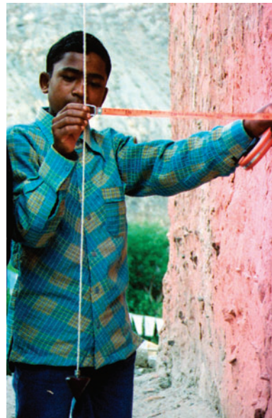
A worker measuring exterior deformation in reference to a vertical plumb line at Chango Temple. Photo: © Sandeep Sikka.
