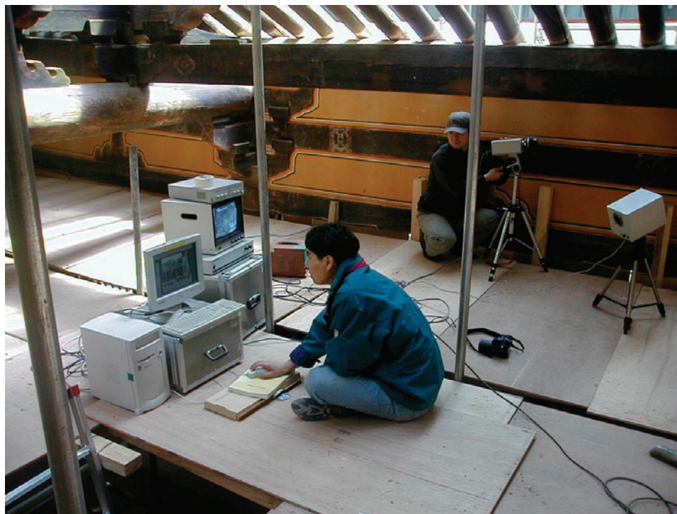
IRR acquisition of the images was conducted both on the individual components and in situ for the composite building. Photo: © Soon-Kwan Kim.
