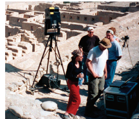
The documentation team at Tambo Colorado preparing to use the Cyrax 2400/2500 (which became the Leica HDS 2500) long-range laser scanner. Photo: © Alonzo Addison.
