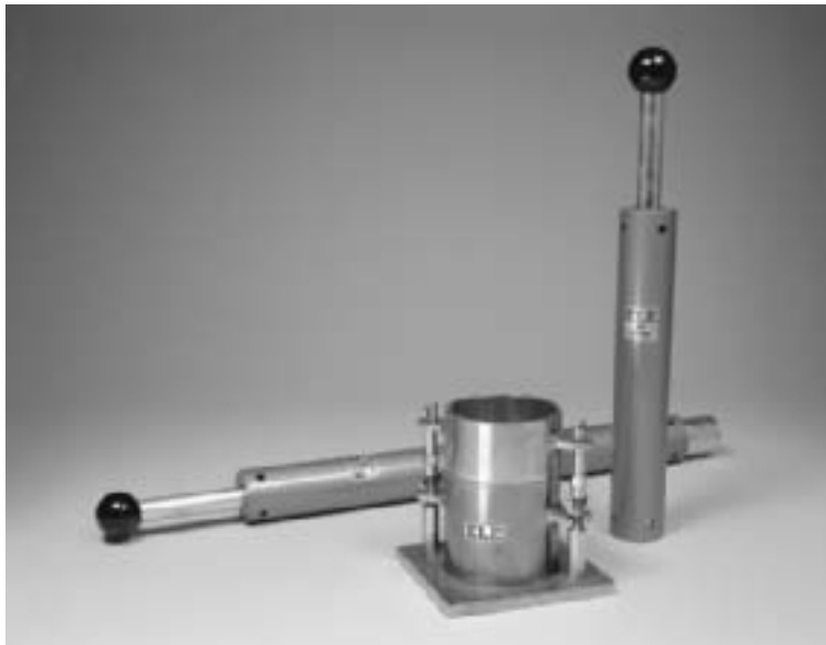
Figure 4.7 Hammer used for the modified Proctor test. (Courtesy of ELE International)
