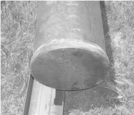
FIGURE 5.3 Closed end of a steel pipe pile.
