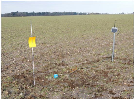
**Fig. 6.7** Field soil moisture monitoring station with an installed capacitance (FDR) soil moisture probe (next to flag at right) and associated solar-powered, radio-controlled telemetry system (fixed to pole at right). (© Kevin Hiscock.)
