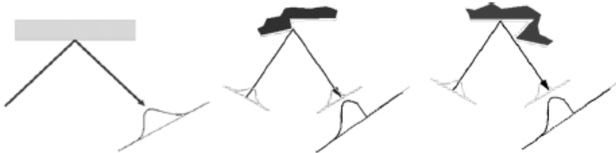
Figure 19 – Ideal reflection, partial illumination, partial occlusion
