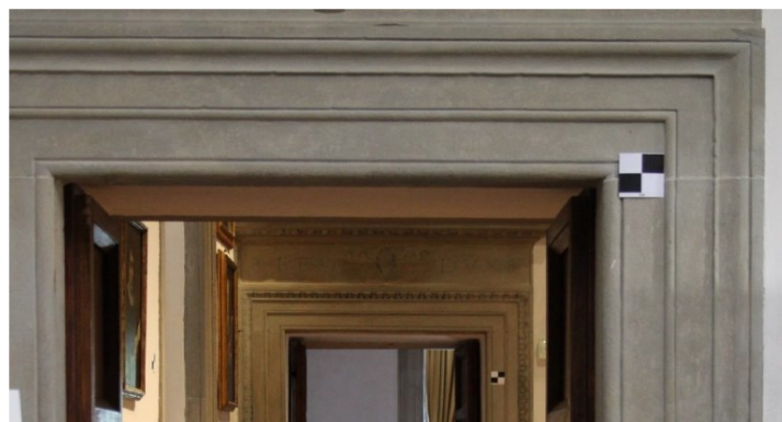
Figure 10 – Marker used both for TLS and Terrestrial Photogrammetry
