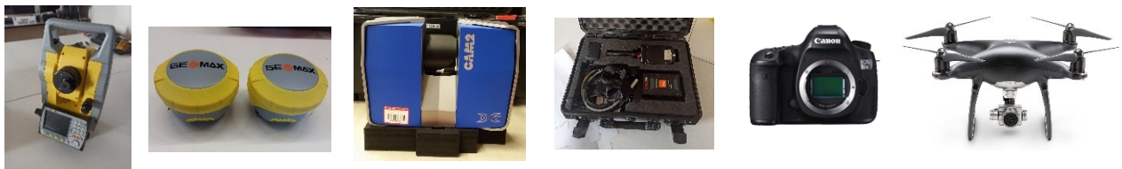
Figure 11 – Set of instruments used for the metric survey: total station, GNSS receivers, Terrestrial Laser Scanner, SLAM-based system, terrestrial digital camera, and a drone equipped with a digital camera.
