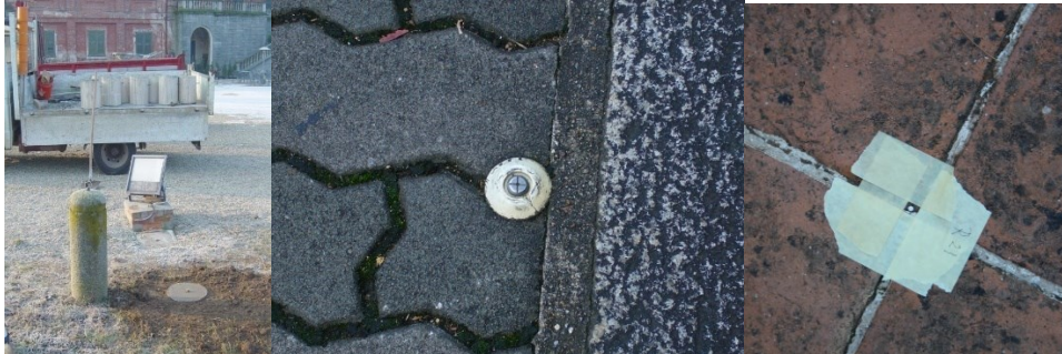
Figure 7 – Permanent materialization of control network's vertexes
