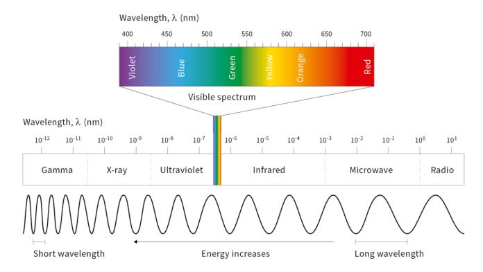
Figure 30 The electromagnetic spectrum.
