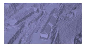
Figure CS4.6 Noisy inputs for the range of buildings on the left resulted in noisy data in that area of the model.
