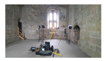
**Figure 27**Lighting rig in use while photographing wall paintings.
