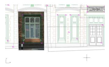
Figure 10 Stages of single image rectification.
