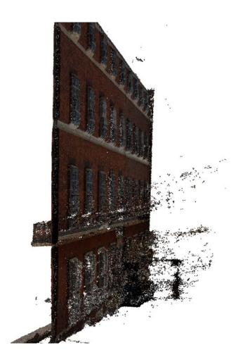
**Figure 77** Extraneous geometry produced when photographing windows.
