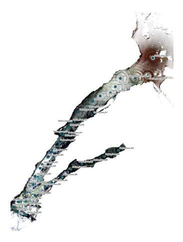
Figure CS4.3 Scanner setups for surveying Merlin's Cave.
