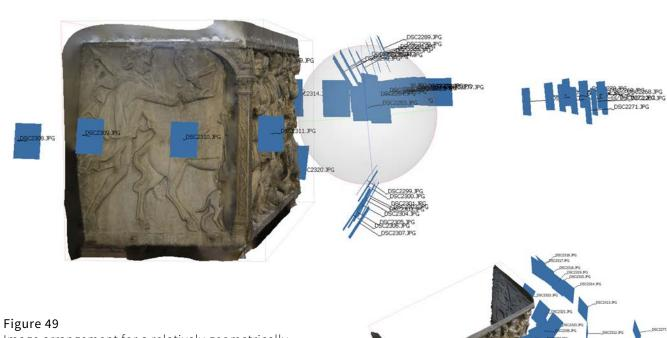
Image arrangement for a relatively geometrically complex carved object.
