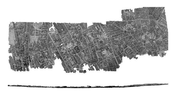
Figure 17 'Bowl' effect caused by inaccurate initial camera calibration estimates. The problem is not immediately visible in plan (top), but the side view (bottom) shows the effect.
