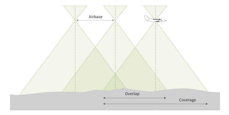
**Figure 34** Forward overlap in vertical aerial imagery.
