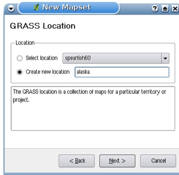
Figure 7.2.: Creating a new GRASS LOCATION or a new MAPSET in QGIS
