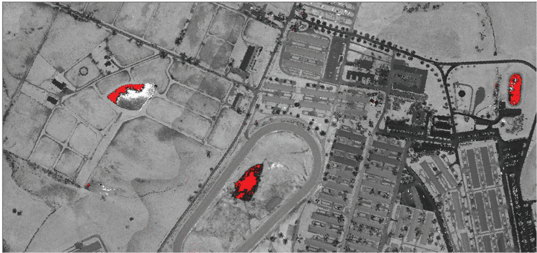
FIGURE 10.6 LiDAR intensity image depicting voids (in red).
