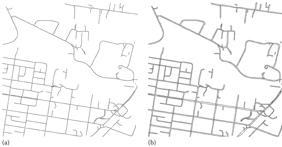
FIGURE 16.18 (a) Vectorized road centerlines and (b) vectorized road edges as calculated from the road centerline and the detected road width. (From Clode, S. et al., Photogram. Eng. Rem. Sens. , 73, 5, 517, 2007. With permission.)
