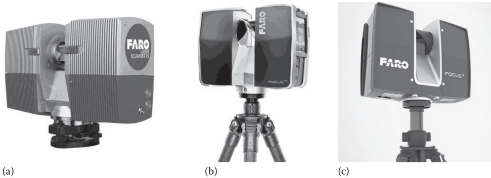
FIGURE 2.7 (a) The earlier FarO LS 420, (b) the later FarO Focus 3D, and (c) the latest FarO Focus S laser scanner, all of which measure their ranges employing phase differences. (Courtesy of FarO. With Permission.)
