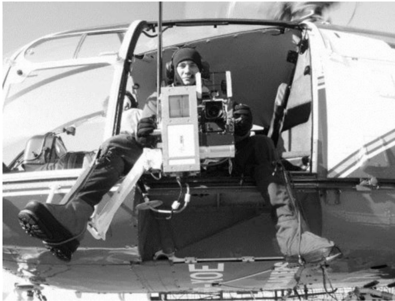
FIGURE 3.27 This example of a Helimap system is being operated from the side of an Alouette III helicopter to measure the steep sides of a valley. (Courtesy of Helimap Systems, Epalinges, Switzerland. With Permission.)
