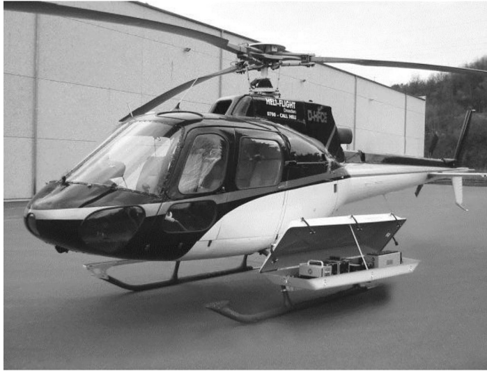
FIGURE 3.25 A helicopter fitted with a specially built Helipod box that is mounted on an outrigger frame and contains an Integrated Geospatial Innovations (IGI) LiteMapper system. (Courtesy of IGI. With Permission.)
