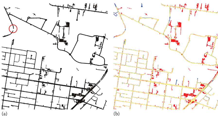
FIGURE 16.14 (a) Results of road network classification. The circle highlights a problem that occurs with bridges. (b) Spatial distribution of the classified pixels. TP pixels are shown in yellow, FP appear in blue, and FN appears in red. (From Clode, S. et al., Photogram. Eng. Rem. Sens. , 73, 5, 517, 2007. With Permission.)
