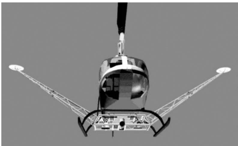
FIGURE 3.29 A helicopter equipped with a FLI-MAP system, which is mounted inside the frame that is attached to the underside of the aircraft; note also the two outrigger pylons, each supporting a GPS antenna. (Courtesy of Fugro, Leidschendam, the Netherlands. With Permission.)
