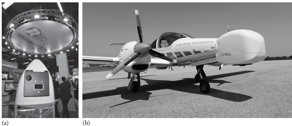
FIGURE 3.24 (a) The universal nose of the Diamond DA42MPP aircraft into which the RIEGL LMS-Q680i laser scanner can be fitted and (b) showing an alternative design of nose cone that has been fitted to a DA42 MPP aircraft. (Courtesy of RIEGL , Horn, Austria. With Permission.)
