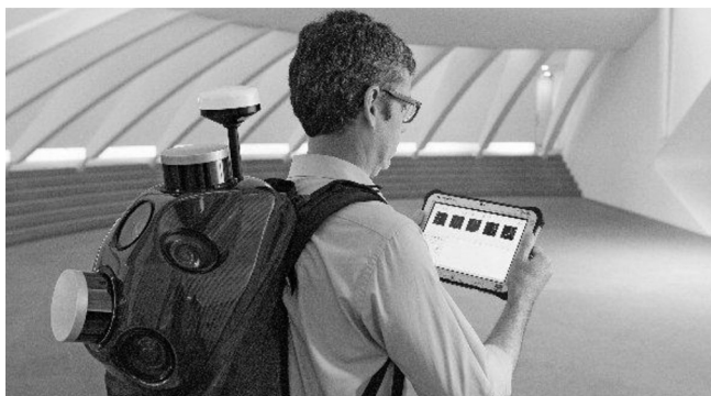
FIGURE 2.53 A Pegasus Backpack mobile mapping system. Note the twin Velodyne Puck profilers, one mounted horizontally, the other vertically; the GNSS receiver; and the ports of three of the small-format digital frame cameras. (Courtesy of Leica Geosystems, St. Gallen, Switzerland. With Permission.)
