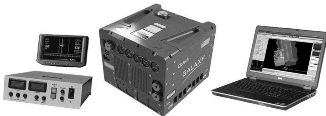
FIGURE 3.13 The principal elements of a Teledyne Optech ALTM Galaxy laser scanning system with the laser scanner unit located at center and the case containing the control electronics at front left. Behind the control box unit is a small display screen that is used in the navigation of the aircraft in-flight, while at right there is a laptop computer that is used for flight management, control purposes, and data storage. (Courtesy of Teledyne Optech, Vaughan, ON. With Permission.)
