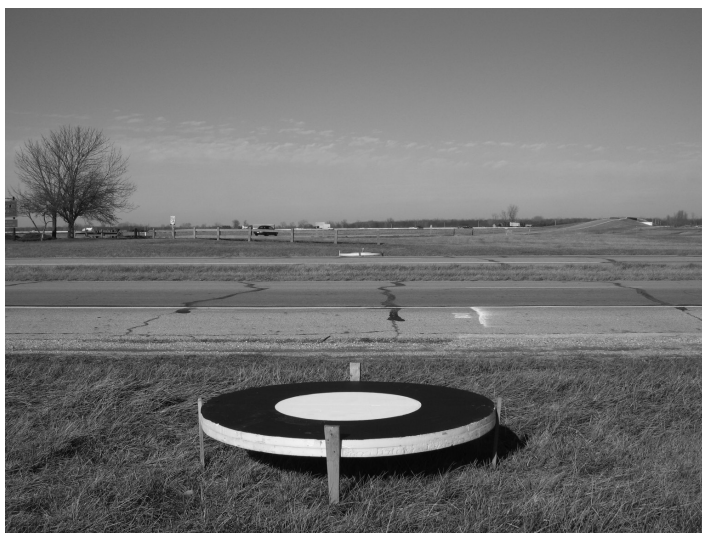
FIGURE 8.4 LiDAR specific ground control point.
