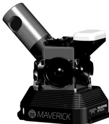
FIGURE 2.41 An Optech Maverick mobile mapping system showing the Velodyne HDL-32 laser scanner/profiler at left and the NovAtel GPS receiver with its white cap at right, with the Point Grey Ladybug5 multiple camera unit placed between them. (Courtesy of Teledyne Optech, Vaughan, ON. With Permission.)
