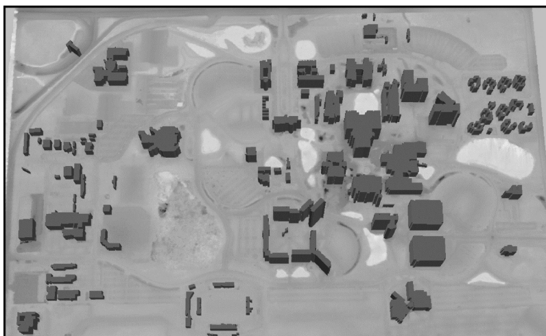
FIGURE 18.10 2.5D building models for FIU campus. Each building model was created using the final footprint and average building height derived from LiDAR measurements. The DTM for building bases was derived by interpolating ground measurements identified by the progressive morphological filter. (From Zhang, K. et al., IEEE Trans. Geosci. Remote Sens. , 44, 9, 2523, 2006. With Permission.)
