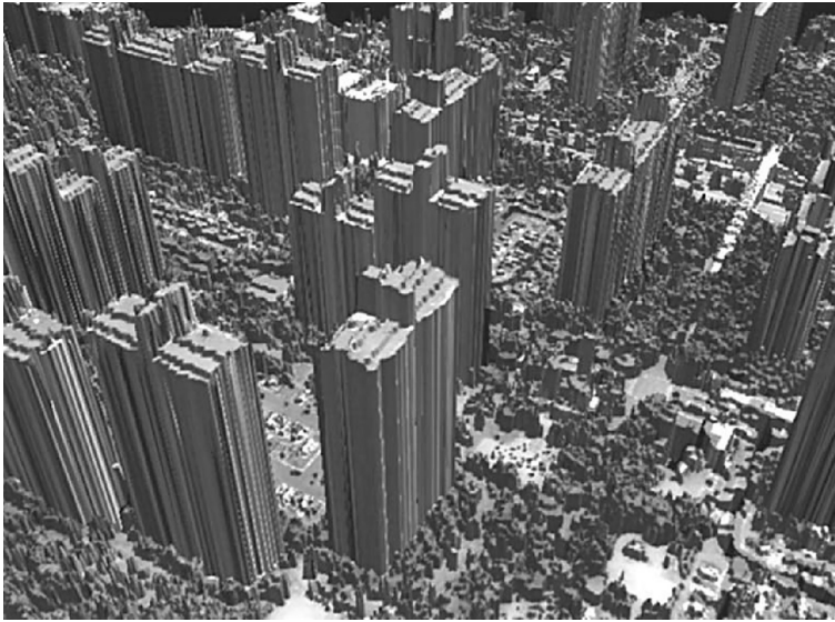
FIGURE 13.27 Photo-realistic 3D model produced by rendering a true orthophoto onto LiDAR data.
