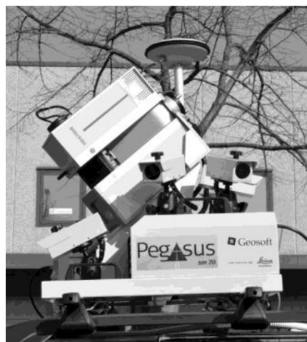
FIGURE 2.51 This Pegasus One system has been fitted with a Leica HDS7000 terrestrial laser scanner with a locked azimuth rotation, so that it acts as a 2D laser profiler. (Courtesy of Leica/Geosoft, Pordenone, Italy. With Permission.)
