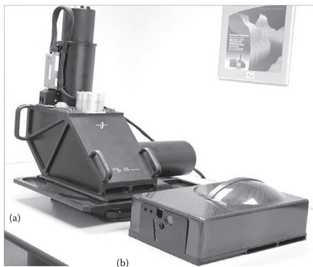
FIGURE 3.16 The difference in size (and weight) between the older Leica ALS40 laser scanner (a) and the newer ALS50 model (b) is quite striking. (Courtesy of Spencer B. Gross, Reno, Nevada. With Permission.)
