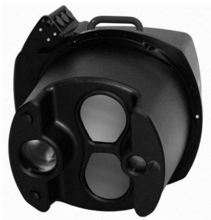
FIGURE 3.56 The Leica-AHAB Chiroptera II airborne bathymetric laser scanner, showing the (larger) twin optical ports installed for the bathymetric and topographic laser scanners respectively and the third (smaller) port for the accompanying digital camera, all located on the underside of the system case. (Courtesy of Leica Geosystems, St. Gallen, Switzerland. With Permission.)
