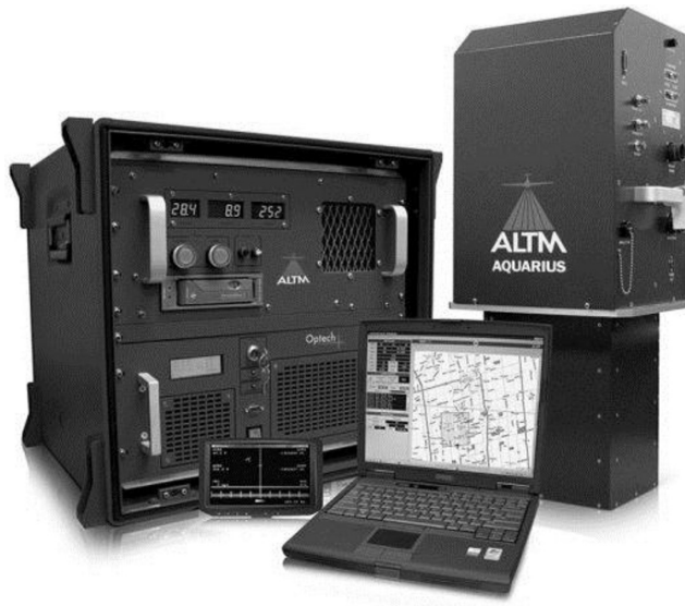
FIGURE 3.55 The Optech ALTM Aquarius shallow-water bathymetric laser scanning system with the laser rangefinder and scanner located at right rear and the control electronics cabinet at left rear. In front is the laptop computer that is used to control the overall system, together with a separate small pilot display monitor. (Courtesy of Teledyne Optech, Vaughan, ON. With Permission.)
