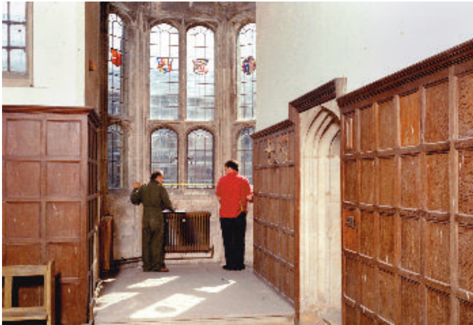
Figure 12 Traditional hand-surveying methods are necessary even where electronic equipment is available. With care they can produce highly accurate results in all but the most difficult conditions. (Apethorpe Hall, Apethorpe, Northants; AA044522)
