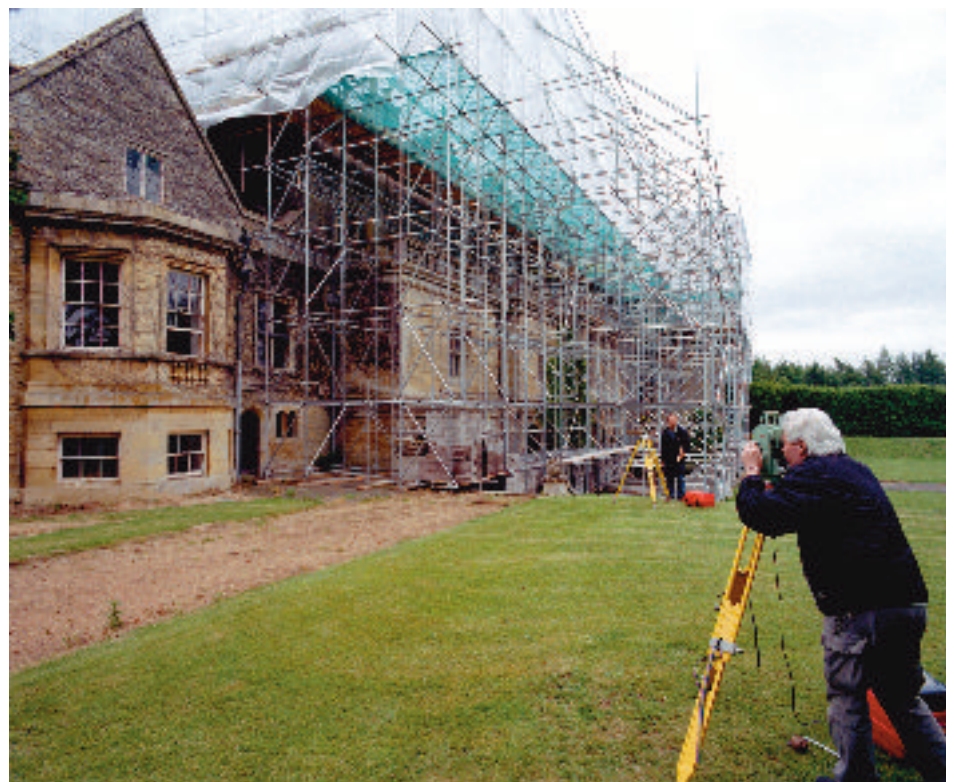
Figure 11 EDM or REDM theodolites can confer immense benefits in both time and accuracy, in surveys of large, complex or irregular buildings, although they cannot make up for poor observation or a lack of understanding. (Apethorpe Hall, Apethorpe, Northants; AA044523)
