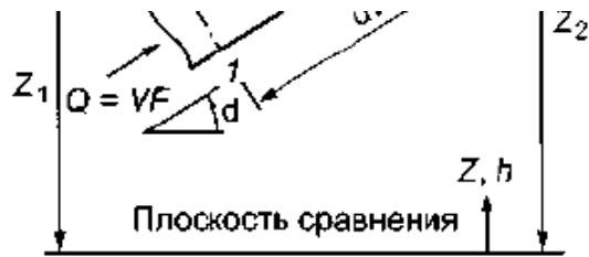
$$Z_1 + \frac{P_1}{\gamma} + \frac{v_1^2}{2g} = Z_2 + \frac{P_2}{\gamma} + \frac{v_2^2}{2g} + \Delta H_{1-2}, \quad (5.5)$$
